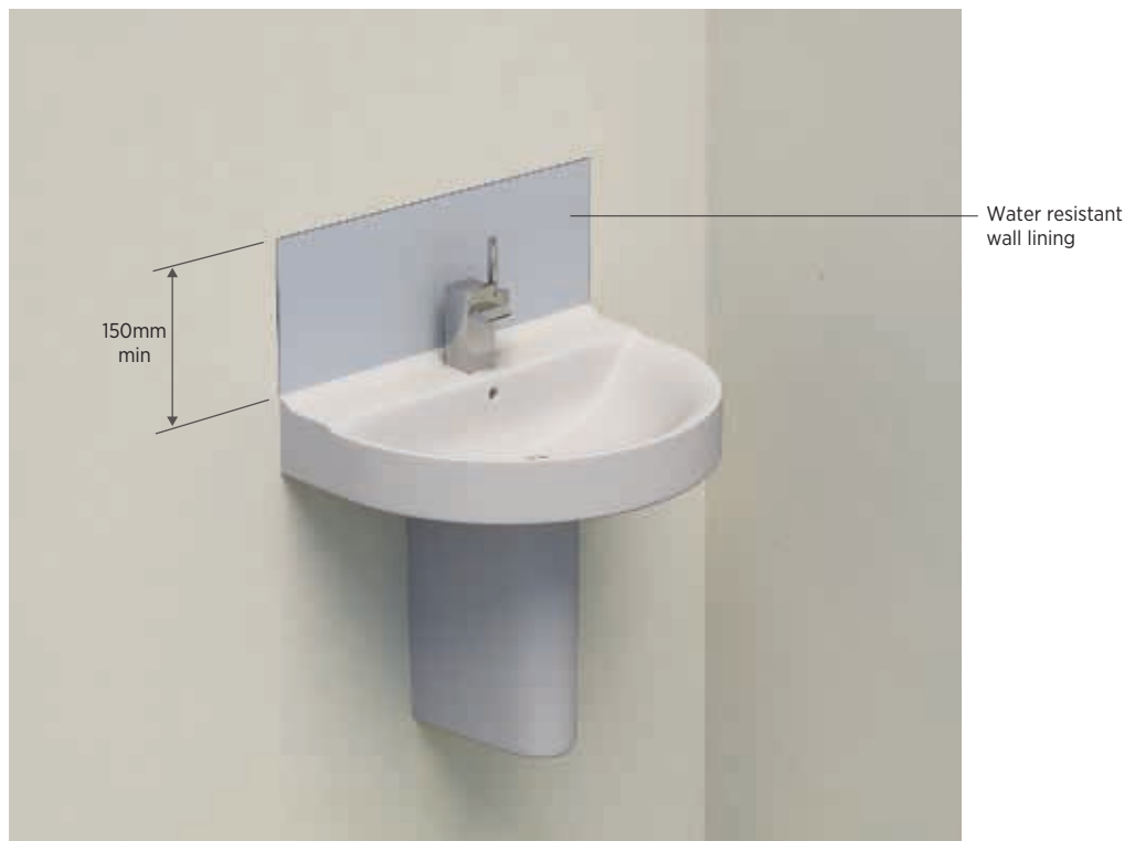
Figure 58: Waterproofing of basin
