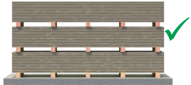
Figure 8: Correct placement of billets
