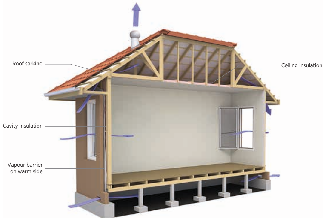
Figure 2: House Ventilation Paths
