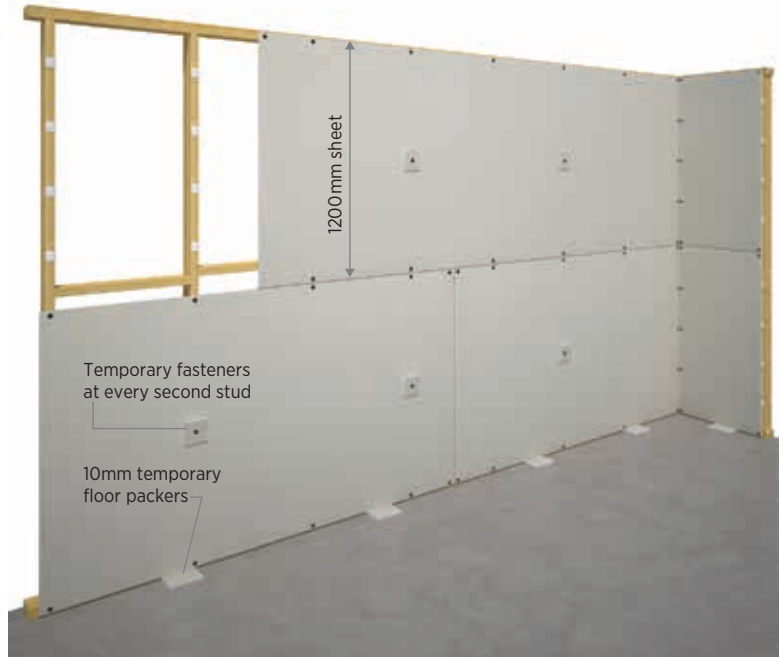
Figure 29: Combination adhesive and screw fixing on walls
